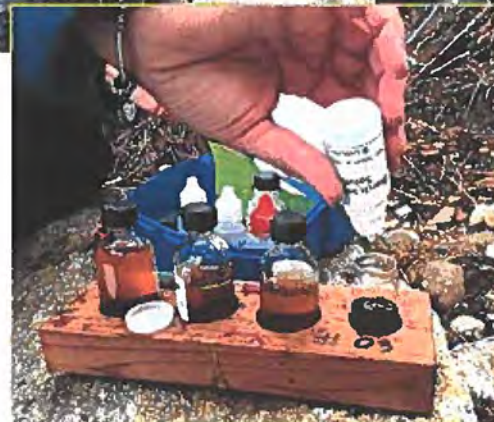
A volunteer uses a titration kit to determine the amount of dissolved oxygen in a sample of water.
